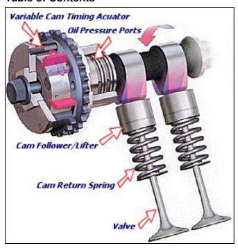
How Camshaft and Variable Valve Timing Works
